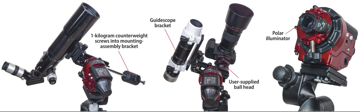
**ASTRO CONFIGURATION #2** The Astro Bundle includes a one-kilogram counterweight for balancing a small 60mm (shown here) to 80mm telescope solidly attached at the end of the declination axis. The telescope will need a mounting shoe with a 1/4-20 tripod socket. The full configuration, sans scope, camera and tripod, weighs 3.7 kilograms.
