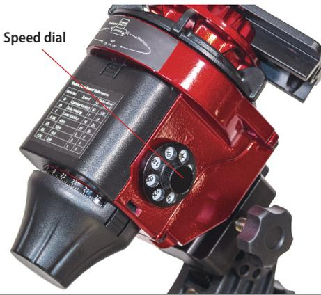
**SPEED CONTROL** The Star Adventurer can turn at the sidereal, solar or lunar rate, as well as at a 0.5x half speed, good for nightscapes to minimize blurring of the ground in tracked shots. The 2x, 6x and 12x speeds are for panning in time-lapse sequences, though only through a preset arc of 60 degrees.
