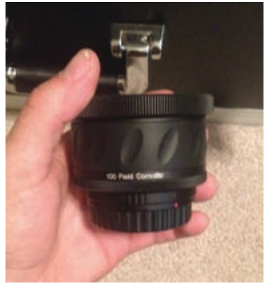
Image 5 - The Esprit 100ED includes a thread-on field flattener.
