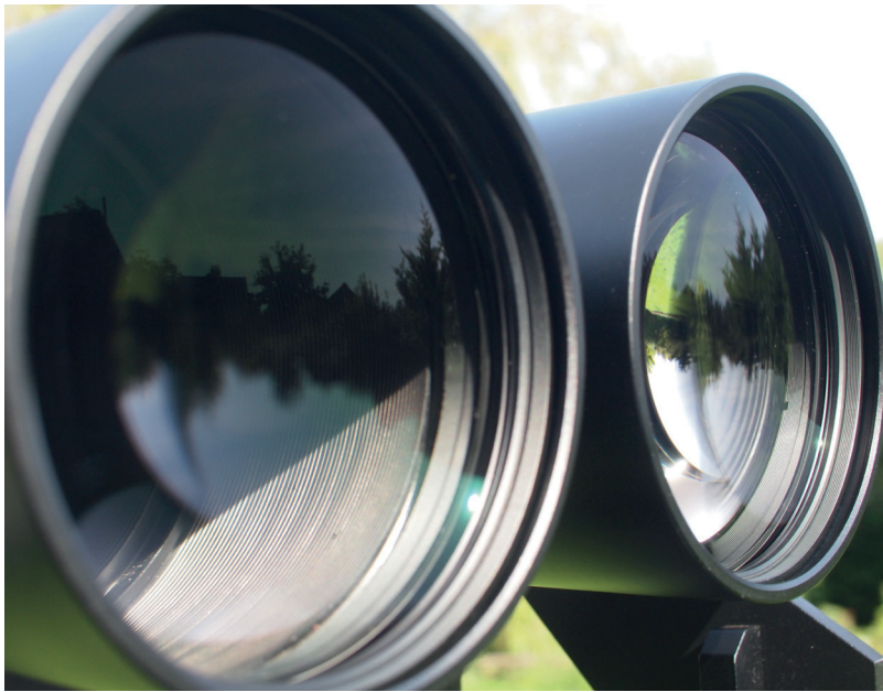
▲ The binoculars' interior surfaces are milled to reduce light scatter. Image: Steve Ringwood.
