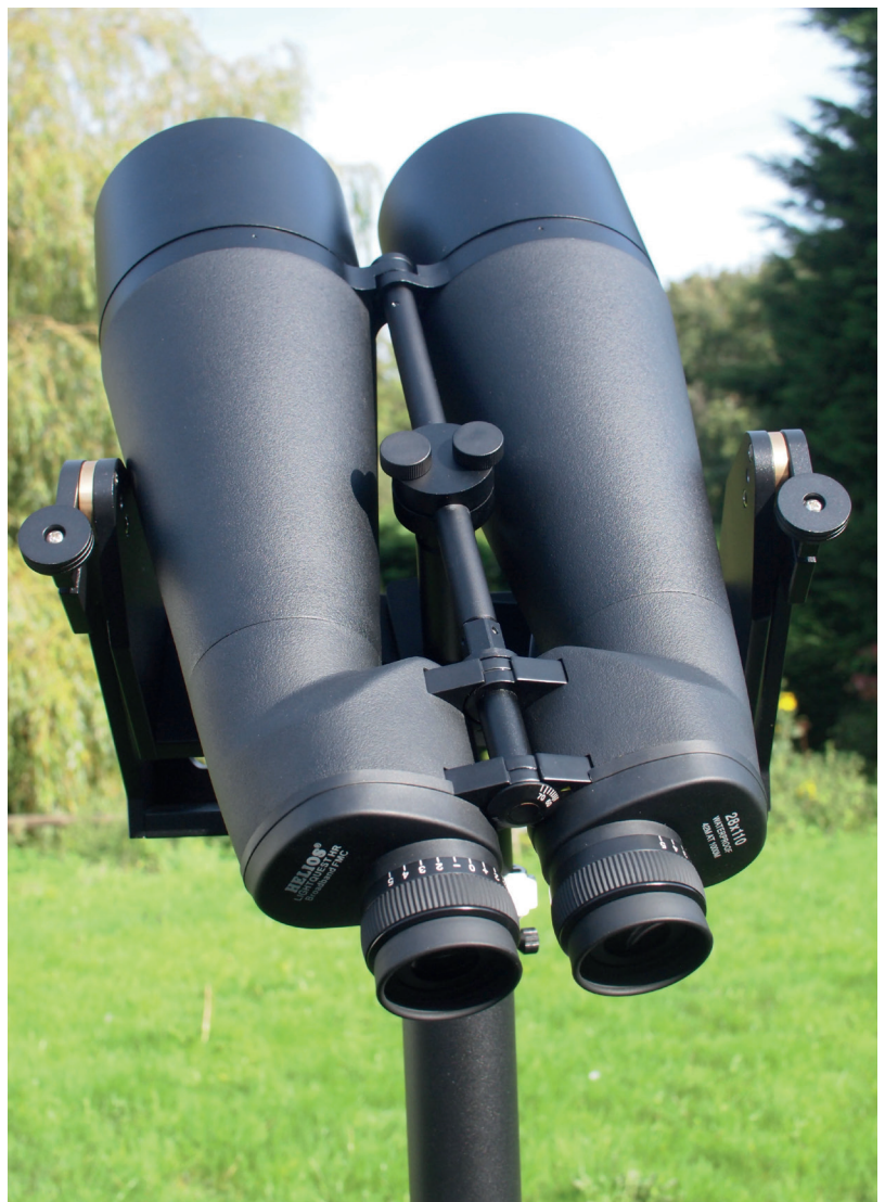
▲ A mount providing room underneath the eyepieces is needed to give access to objects at the zenith. Image: Steve Ringwood.
