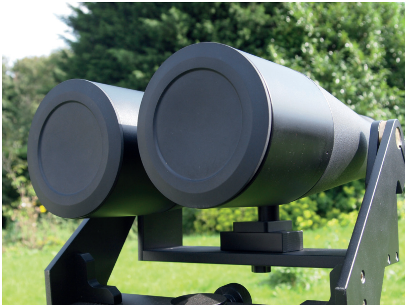
▲ The object lenses are hermetically protected by rubber caps – be careful not to break finger nails trying to pry them off! Image: Steve Ringwood.
