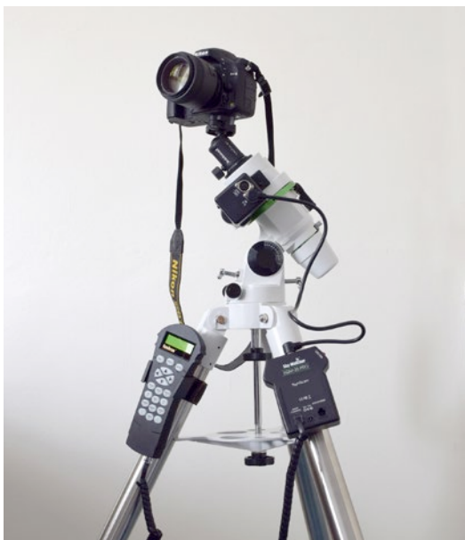
▲ The cable for flashing (i.e. upgrading/overwriting) the SynScan firmware has an RS 232 connector, which is not found on many modern computers. Image: Geoffrey Lenox-Smith.
