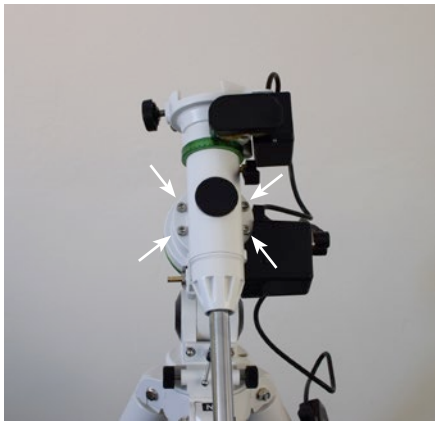
▲ Removing the dec. head from the EQM-35 for travel mode, which highlights the modular aspect of the mount. First, take off the dec. body by unscrewing the four M6 bolts (arrowed) using an Allen key. This exposes the mount head, onto which the saddle head can then be installed using the four M5 bolts provided. Images: Geoffrey Lenox-Smith.
