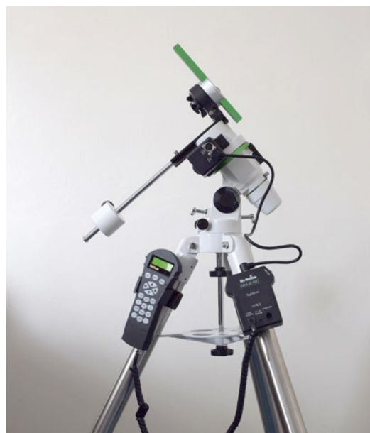
◀ The EQM-35 mount in its 'light' travel mode, with the dec. bar removed and using components from the Star Adventurer Astro bundle. Image: Geoffrey Lenox-Smith.
