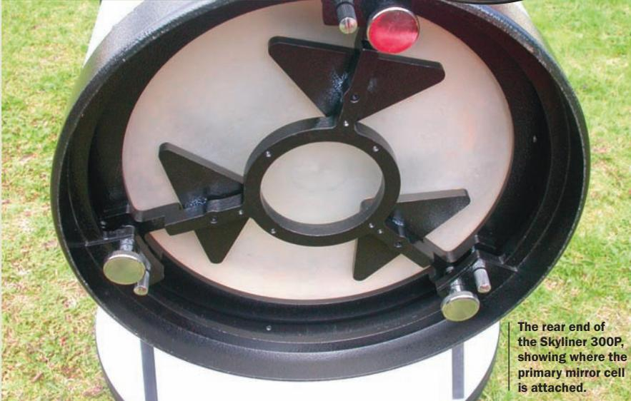
The rear end of the Skyliner 300P, showing where the primary mirror cell is attached.
