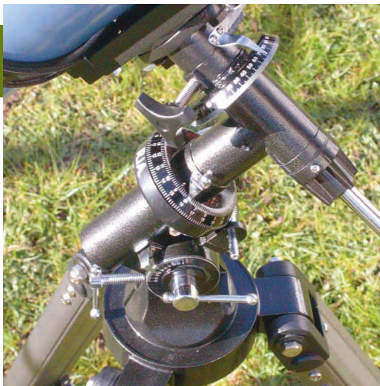
Left: The EQ2 German equatorial mount sports setting circles and slow motion controls on both axes. A relatively lightweight mount, it handles the Explorer-130PM tube assembly with ease. Vibration damping time is in the region of three seconds.
