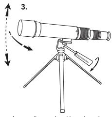
Loosen the pan head lever to make side-to-side or up-and-down adjustments.
