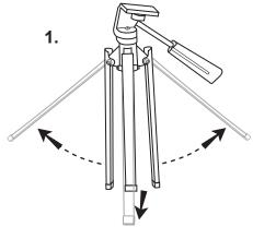
Spread tripd legs completely and set on firm support.
