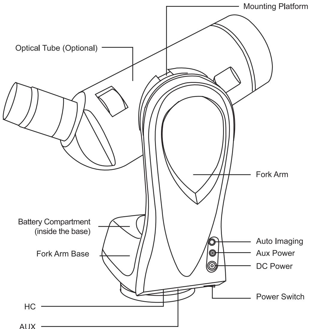
**Auto Imaging** — Electronic shutter interface. This controls software action from the mount to devices such as digital spotting scope or Canon EOS digital cameras.
