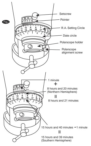
magnitude star Vega in the Constellation Lyra. From a star chart we know the R.A. coordinate of Vega is 18h 36m. Loosen the R.A. and DEC. lock knobs on the mount and adjust the telescope so that Vega is centred in the field of view of the eyepiece. Tighten the R.A. and DEC. lock knobs to lock the mount in place. Now rotate the R.A. setting circle until it reads 18h36m. You are now ready to use the setting circles to find objects in the sky.
