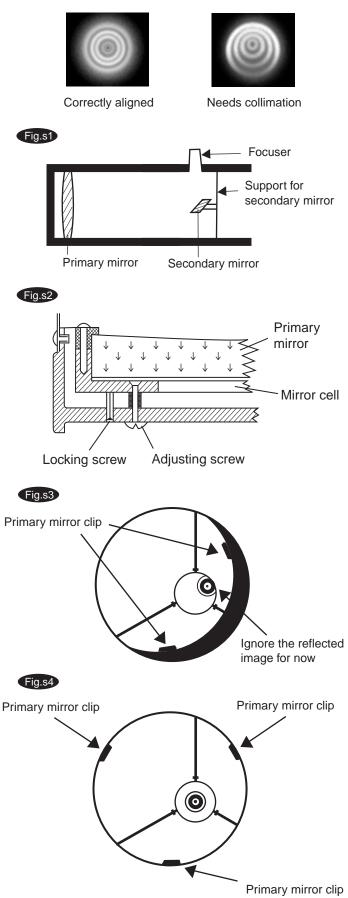
alternately loosen one and then compensate for the slack by tightening the other two. Stop when you see all three mirror clips (Fig.s4). Make sure that all three small alignment screws are tightened to secure the secondary mirror in place.
