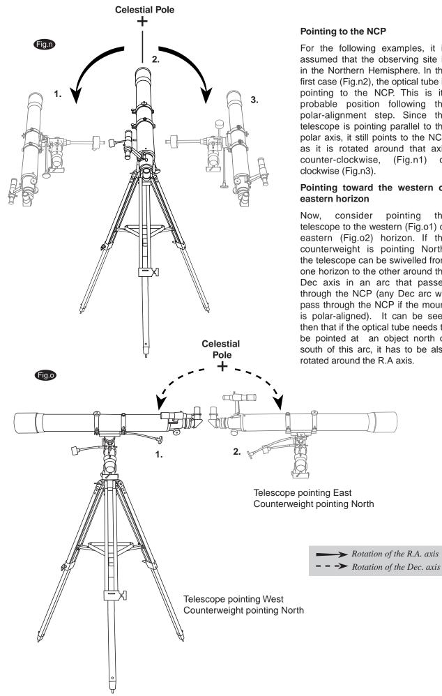
For the following examples, it is assumed that the observing site is in the Northern Hemisphere. In the first case (Fig.n2), the optical tube is pointing to the NCP. This is its probable position following the polar-alignment step. Since the telescope is pointing parallel to the polar axis, it still points to the NCP as it is rotated around that axis (Fig.n1) or
