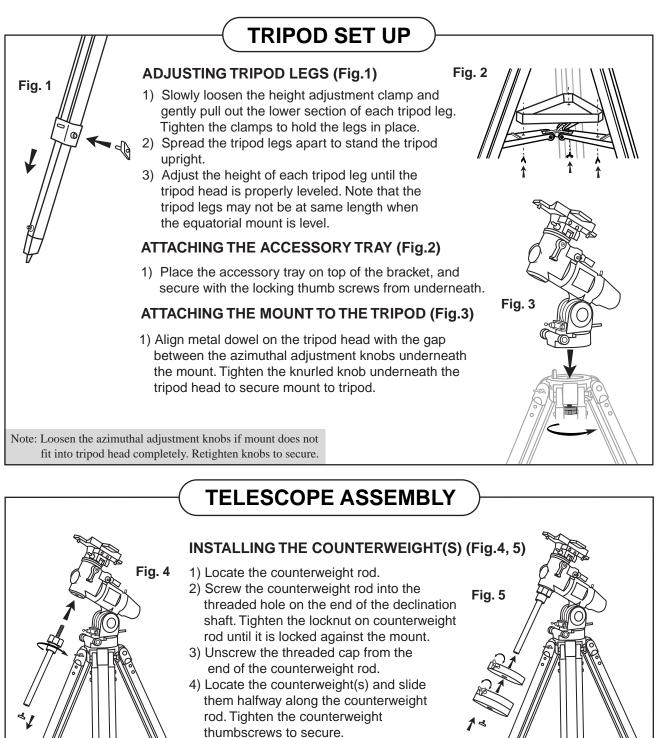
5) Replace the cap on the end of the counterweight rod.
