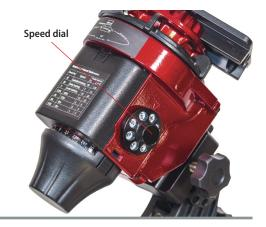
**SPEED CONTROL** The Star Adventurer can turn at the sidereal, solar or lunar rate, as well as at a 0.5x half speed, good for nightscapes to minimize blurring of the ground in tracked shots. The 2x, 6x and 12x speeds are for panning in time-lapse sequences, though only through a preset arc of 60 degrees.
