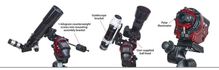
**ASTRO CONFIGURATION #2** The Astro Bundle includes a one-kilogram counterweight for balancing a small 60mm (shown here) to 80mm telescope solidly attached at the end of the declination axis. The telescope will need a mounting shoe with a ¼-20 tripod socket. The full configuration, sans scope, camera and tripod, weighs 3.7 kilograms.
