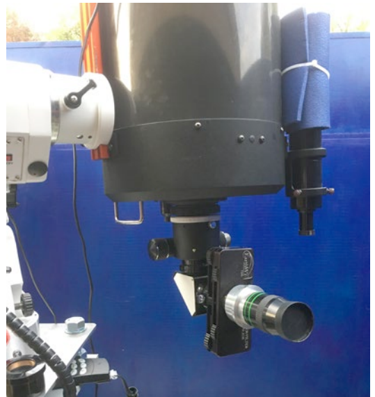
▲ Even when tilted at a vertical angle, the focuser retains its firm lock.
