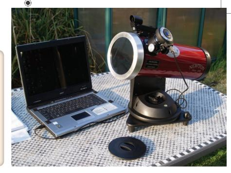
▲ The telescope hooked up to an Orion Solar System imager with a glass aperture filter for a spot of solar observing.
