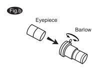
In addition to increasing magnification, the benefits of using a Barlow lens include improved eye relief, and reduced spherical aberration in the eyepiece. For this reason, a Barlow plus a lens often outperform a single lens producing the same magnification. However, its greatest value may be that a Barlow can potentially double the number of eyepiece in your collection.
